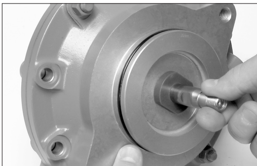
Figure 34 - Checking stem for free movement
