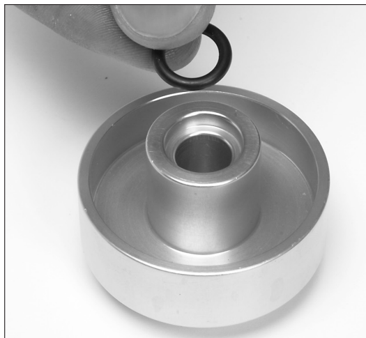
Figure 31 - Fig. 31 Inspecting stem o-ring
