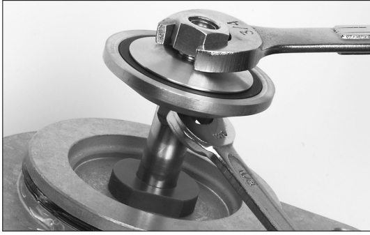
Figure 51 - Remove the stem nut
