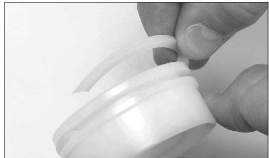
Figure 37 - Installing piston ring on piston
