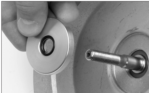
Figure 32 - Installing lower diaphragm retainer
