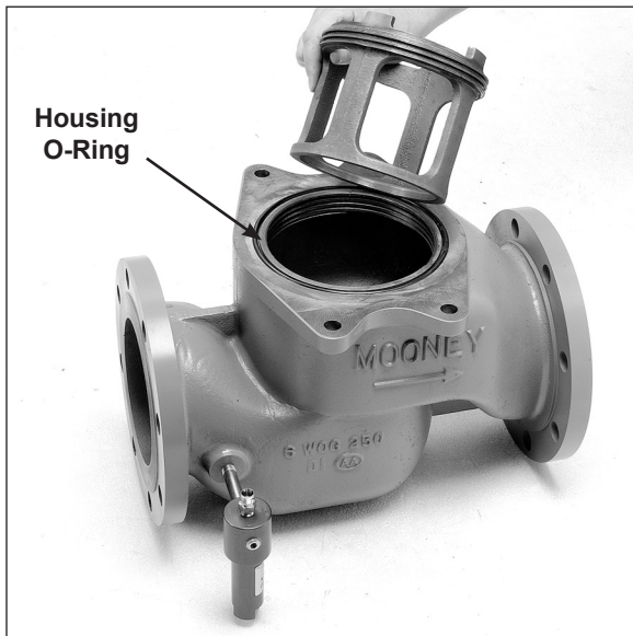
Figure 7b - 6" FlowMax: remove cage & inspect housing o-ring
