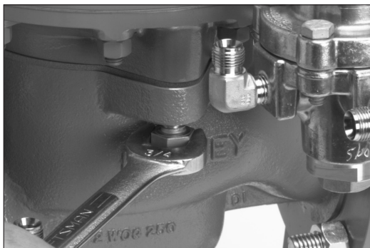
Figure 43 - Tightening the body cap screws
