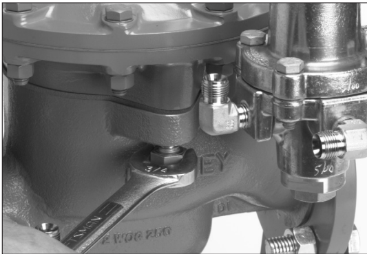
Figure 17 - Tightening the body cap screws
